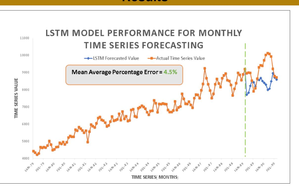
The last 18 data points have been forecasted using LSTM for 1400 monthly univariate time series.
